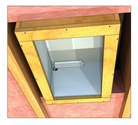
Run the wire through the boxes. Bend the wires so the wires won't slip back through the hole in the box.
