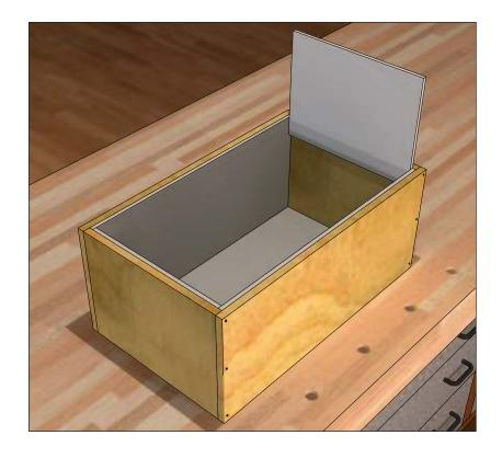
Install the bottom and the four sides of the to the OSB/Plywood box. Screw Cement Board into place compressing the Green Glue between the OSB/Plywood and Cement Board.
