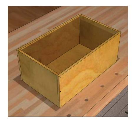
The outside of box is built first, made from 7/16" OSB or plywood. Screw the panels together.
