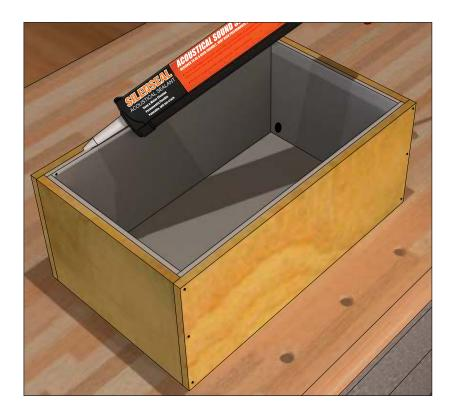
Apply SilenSeal Acoustical Sealant around the top edge of the box.
