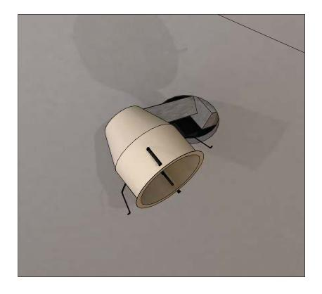
Connect electrical wiring to light-can's junction box. Follow manufactures specifications for installation.
