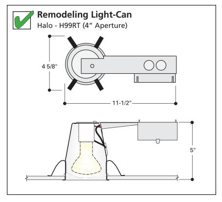
The remodel light-can will be secured to the drywall. The Backer Box will be secured to the ceiling drywall, eliminating any flanking path.
