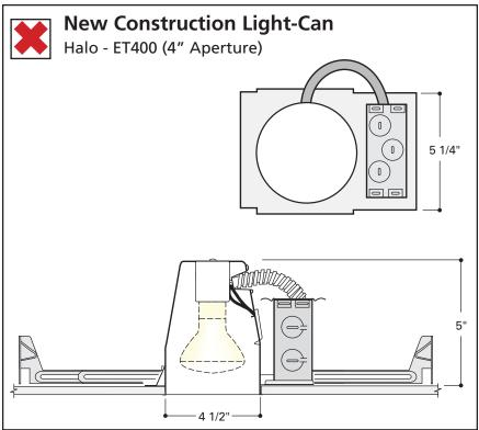
The telescoping arms of the new Construction-Light will allow sound to travel into the ceiling joists. We want to avoid this.
