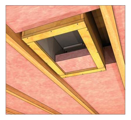
Add a small amount of fiberglass insulation (no paper face) into the box. The location isn't a concern, but some absorption in the box to reduce resonance is preferred.
