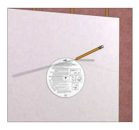
When you are ready to install the ceiling drywall, pre-mark the holes for the ceiling-can. Use the manufactures template to acquire a tight fit. Double check with a dry fit and then cut the hole before installing the drywall.
