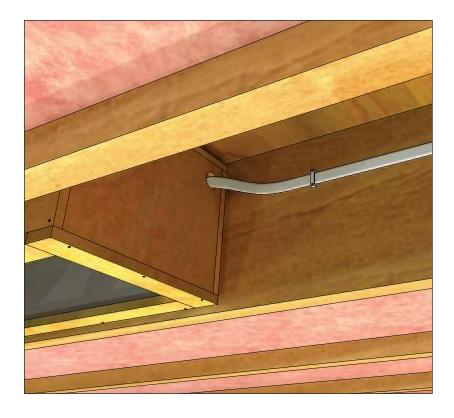
Run electrical wire according to local building codes. Leave the wire 24" longer than necessary inside the box.
