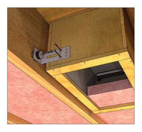
You can use a DC-04 Clip to secure the box to the joist. This will allow your Backer Box to remain in position without creating an additional flanking path. If your budget allows, this will help ease installation of finished drywall. (Make sure the Backer Box is installed at the same height of your joists or furring channel. The Backer Box needs to sit tight to the drywall.)
