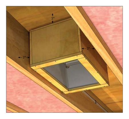
The Backer Box cannot contact any original framing, pipe, duct, etc.
