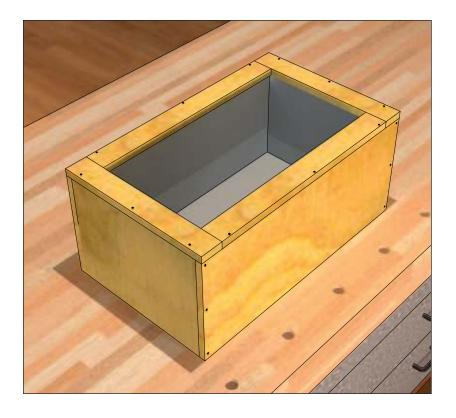
Add a small nailing flange to the box. That flange will accommodate the SilenSeal Acoustical Sealant later.
