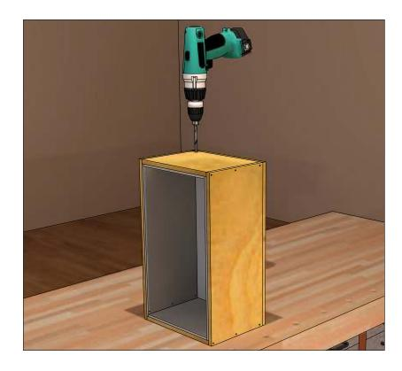
Drill access hole for the electrical wiring. Make the hole just large enough to thread the wiring. Later we will seal this hole with SilenSeal Acoustical Sealant or Putty Pad.
