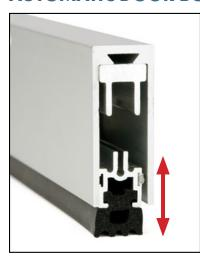
This will seal the bottom of the door. The Neoprene bottom deploys downward when the door is closed. When the door opens, the Neoprene retracts back up into the aluminum housing.
