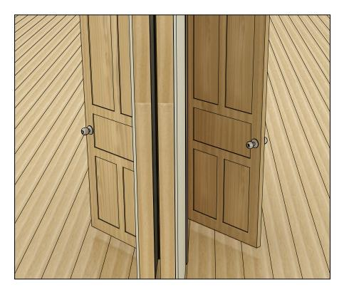
You will need to accommodate the protrusion of both door handles.
