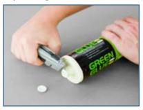
Use a utility knife and cut opening in the Green Glue tube. Tighten nozzle to opened Green Glue tube.
