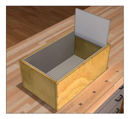
Install the bottom and the four sides of the Cement Board to the OSB/Plywood box. Screw Cement Board into place compressing the Green Glue between the OSB/Plywood and Cement Board.
