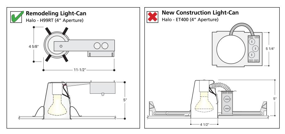
The remodel light-can will be attached to the drywall. The Backer Box will be sealed to the top surface of the ceiling drywall, eliminating any flanking path. The telescoping arms of the new Construction-Light will allow sound to travel into the ceiling joists. We want to avoid this.
