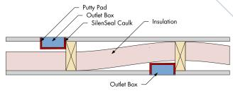
Note that outlets are placed in different wall cavities
